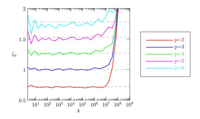
scale very much like experimental structure exponents for 3D turbulence (dashed lines) [Herweijer & van de Water 1995].
